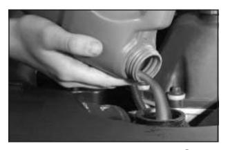
3. Fill the radiator with the proper DEX-COOL® coolant mixture, up to the base of the filler neck. See *Engine Coolant on page 5-24* for more information about the proper coolant mixture.
